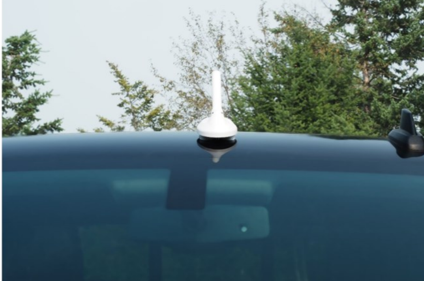
VTU-20 VMAT External Enclosure with Integrated Antenna Assembly
